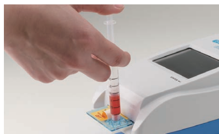
STEP 2 Inject a blood sample to the injection inlet. INJECT
